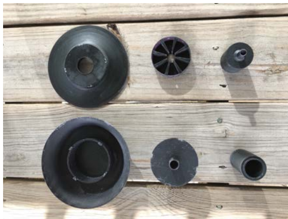
Figure 47. Exploded View of Six Component 3D Printed Inlet
