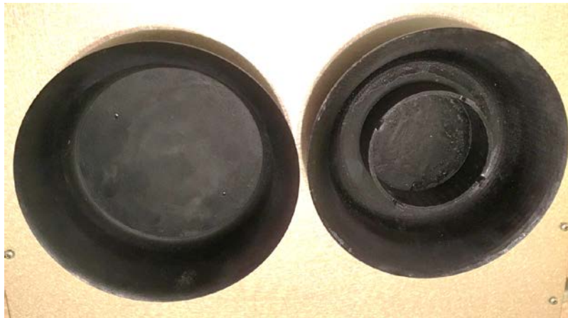
Figure 53. Side-by-side comparison of initial design (left) and revised design (right) of Bell Cap
